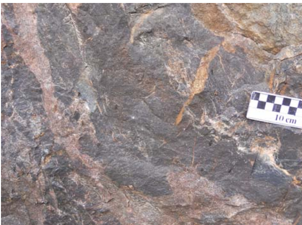
Figure 5. Magnetite-hematite ore (dark) in contact with apatite-carbonate-quartz rock (reddish) in the Nukutus deposit.
