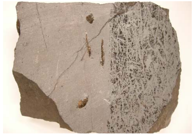
Figure 6. Massive magnetite ore with voids and sharp contact to skeletal magnetite in the Henry deposit. View 15 cm across.
