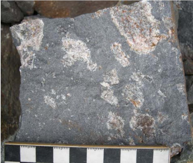
Figure 4. Magnetite-hematite ore with blebs of carbonate, apatite, and quartz in the Nukutus deposit. Scale in cm.
