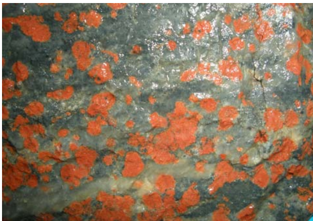
Figure 2. Silicified rhyolite with spots of red K-feldspar. Rektorn hanging wall. View 10 cm across.
