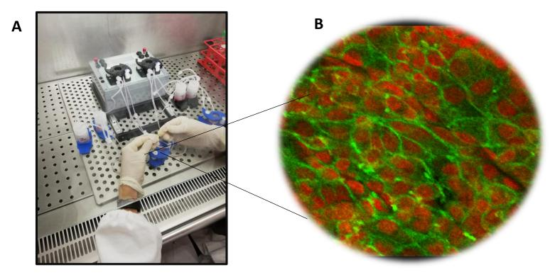
(A) the LB2 biorector connected to perystaltic pump.
